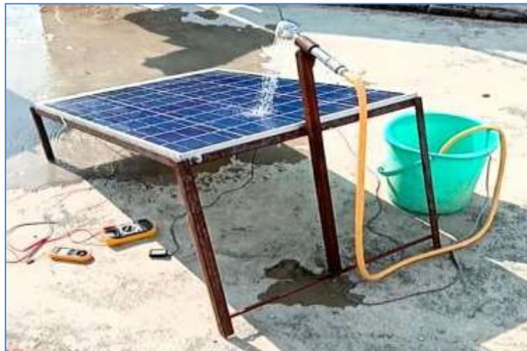
Figure 2. Photograph of Solar Panel Water Spray Cooling System
