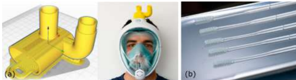
Figure 3(a) 3D printed emergency respirator valve by Isinnova and Weerg [5], reproduced with permission from Isinnova, and (b) NP swabs additively fabricated by Origin using SLA method [6].
