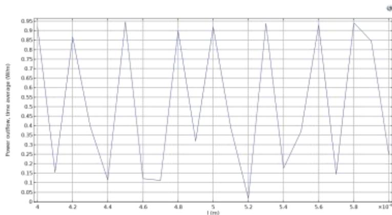
Figure 5 Power outflow (W/m) at port D with variation of distance between the rings L from  $1 \mu\text{m}$  to  $2.5 \mu\text{m}$  with step size of  $0.1 \mu\text{m}$ .
