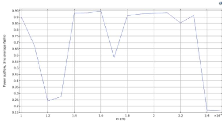
Figure 4 Power outflow (W/m) at port D with variation of ring radius R from  $1 \mu\text{m}$  to  $2.5 \mu\text{m}$  with step size of  $0.1 \mu\text{m}$ .
