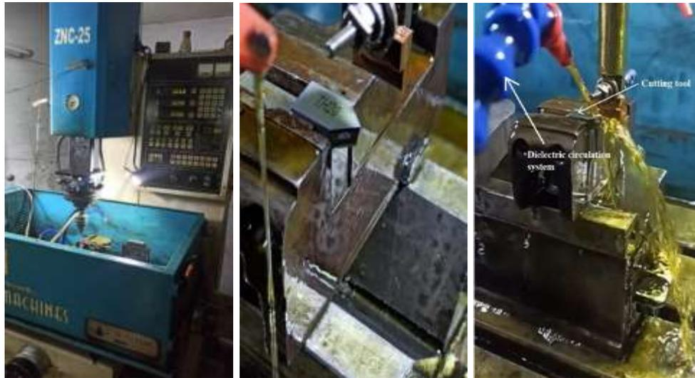
Figure 2. Texturing performed on EDM
