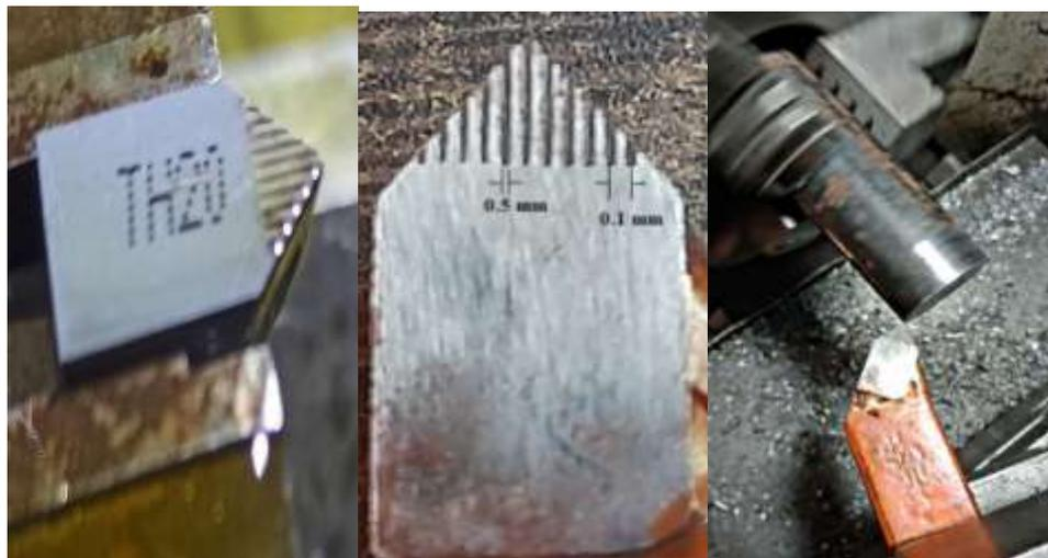
(a) Parallel textures produced by EDM; (b) Dimensions of parallel texture (c) Turning performed on AISI 4340 by parallel textured cutting tool
