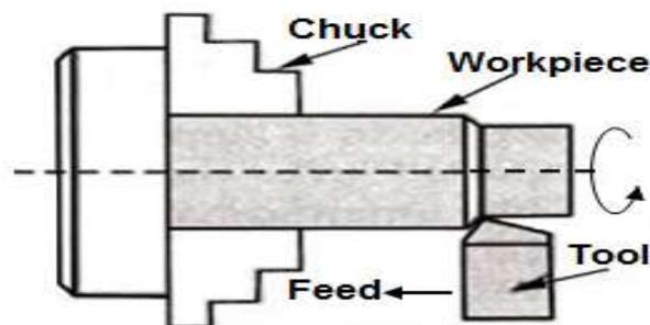
Figure 1. Turning process [1]
