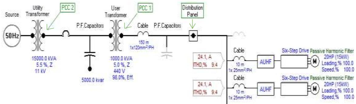
Figure 3.3. Single line configuration for simulating scenario 3
