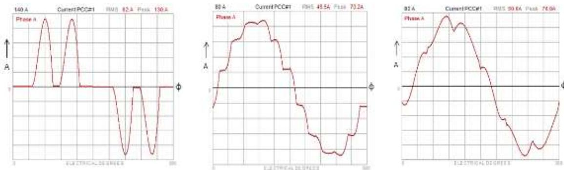
Figure 4.1. Total harmonic current waveforms of scenarios 1, 2 & 3 respectively
