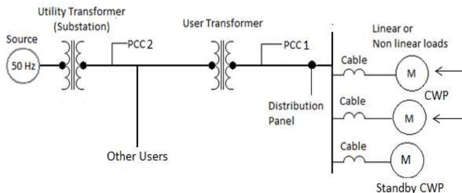
Figure 2.2. Single line diagram showing power distribution system
