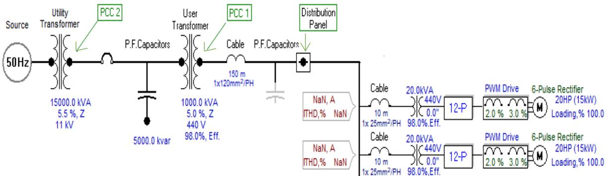
Figure 3.2. Single line configuration for simulating scenario 2
