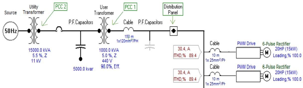
Figure 3.1. Single line configuration for simulating scenario-1
