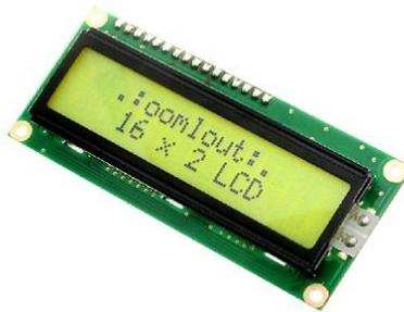
LCD display is used in showing current status of the system output
