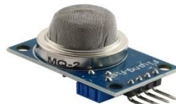
Fig 2. MQ - 2 CO Gas Detection Sensors
