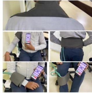
Fig: 12 Prototype of Proposed Massage Band Fig: 13 Applying at different Parts in a body
