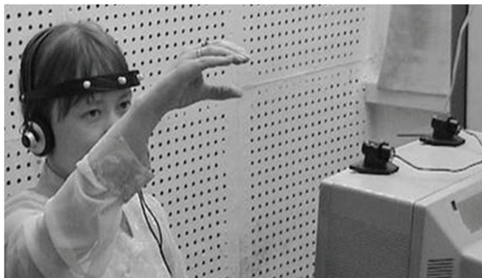
Figure 5.10 Training with the use of a system for the recognition of hand movements and gestures without "Sensitized Gloves" against the real background of the operator's work station.
