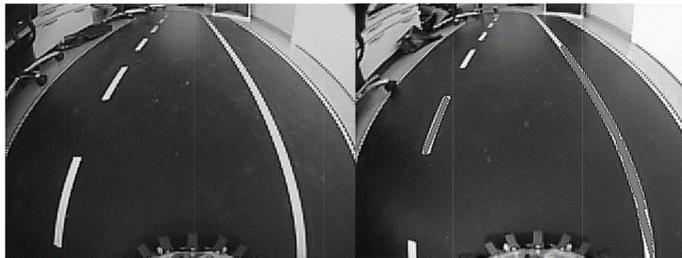
**Figure 9.8** Original image without and with Hough-lines.
