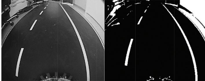
**Figure 9.7** Comparison between original and in-range image.
