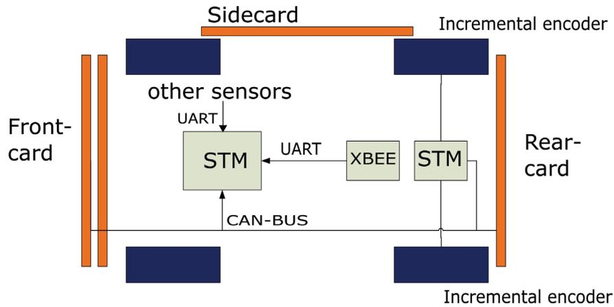
**Figure 9.6** Overview of the data processing system.
