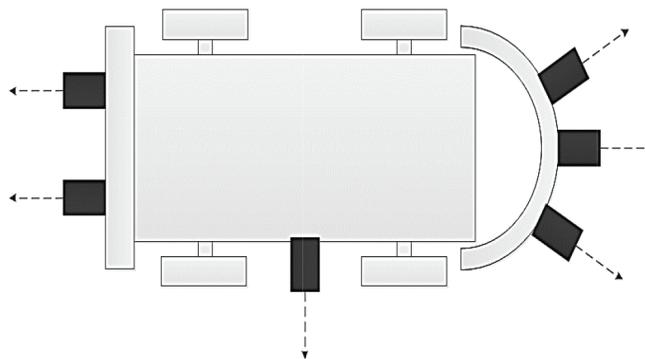
**Figure 9.3** The infrared sensors distributed alongside the car.
