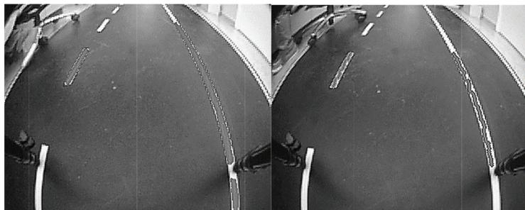
**Figure 9.9** Hough-Lines and sorted points along the Hough-Lines.
