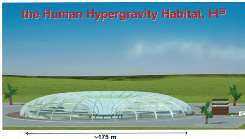
**Figure 11.2** View of the outside structure that accommodates the envisaged human hypergravity habitat ( $H^3$ ). The  $H^3$  is a large-diameter ( $\sim 175$  m) ground-based centrifuge where subjects can be exposed to higher  $g$ -levels for periods up to weeks or months. The  $H^3$  can be used in preparation for future human exploration programs as well as for regular human physiology research and applications [26, 27]. (Image © BERTE bvba/van Loon et al. 2012).
