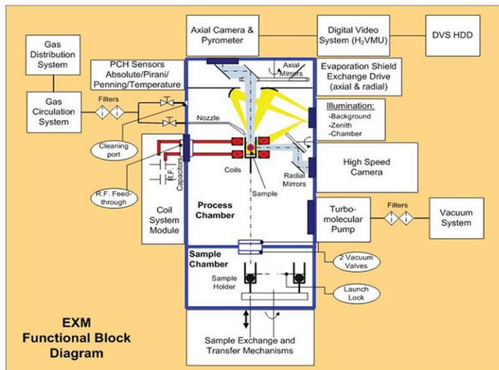
**Figure 21.6** Schematic presentation of (a) the Materials Science Laboratory, and (b) the electromagnetic levitator reaching temperatures up to 2200 C.
