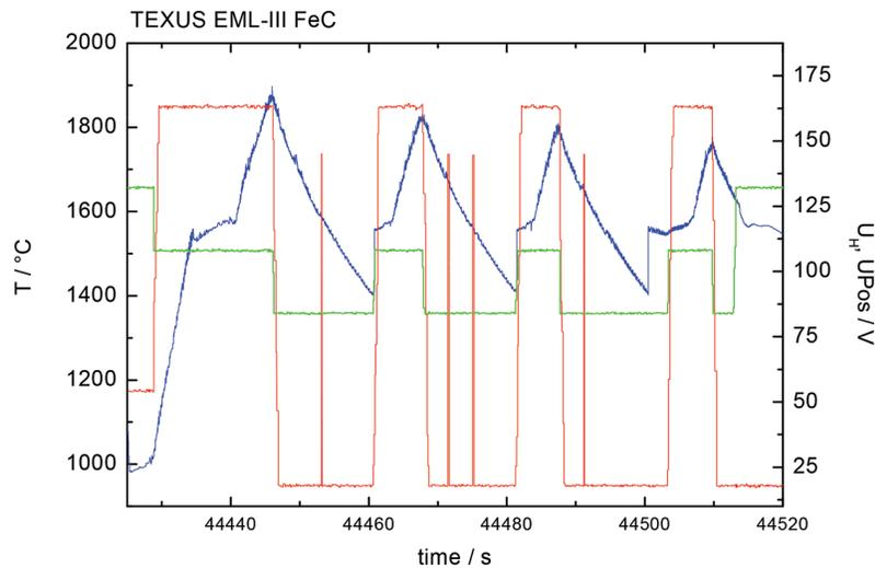
**Figure 21.5** Temperature-time profile of Fe-C alloys processed on the TEXUS 46 EML-III sounding rocketed flight with temperature scale (left) and heater and positioner voltage (right ordinate).
