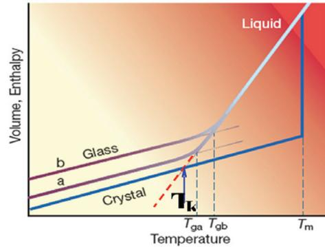
**Figure 21.2** Volume and enthalpy of a glass-forming alloy as a function temperature and undercooling.
