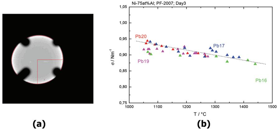
**Figure 21.4** (a) Video image of a fully spherical liquid sample of a NiAl alloy in EML obtained on a parabolic flight for surface tension and viscosity measurements of liquid metallic alloys, (b) Surface tension of a drop of molten Ni-75 at.% Al.
