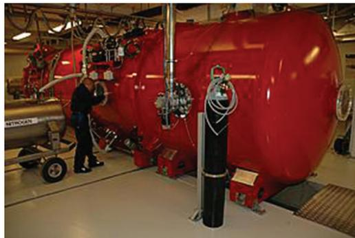
**Figure 5.4** The Aarhus wind tunnel simulator. *Image credit* Mars Simulation Laboratory, Aarhus University.
