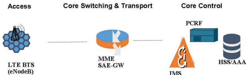
**Figure 10.6** LTE/SAE system architecture (Picture NSN).
