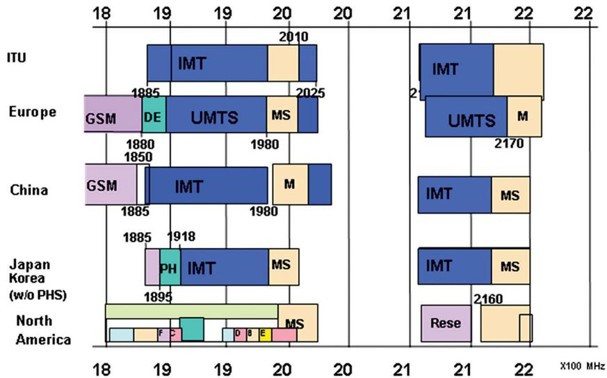
Figure 10.4 IMT 2000 worldwide frequency plans (Picture Siemens).
