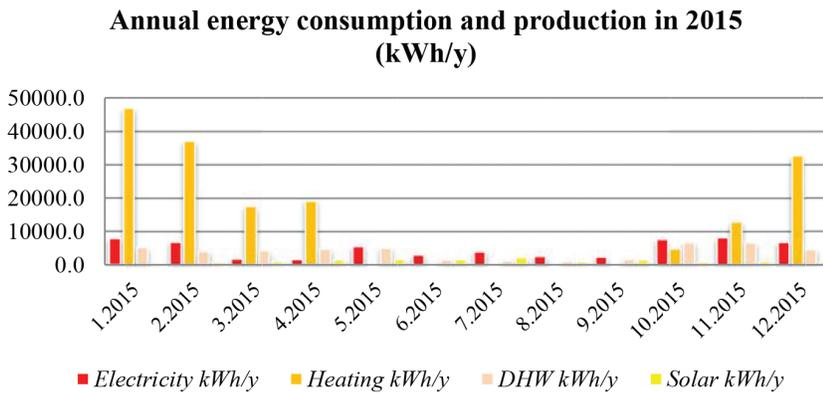
**Figure 8.4** Monthly energy consumption in 2015 (kWh/y).
