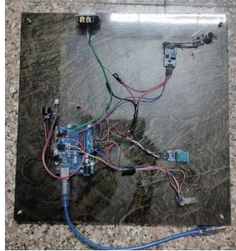
Fig. 7 overall assembly of the proposed smart baby cradle system
