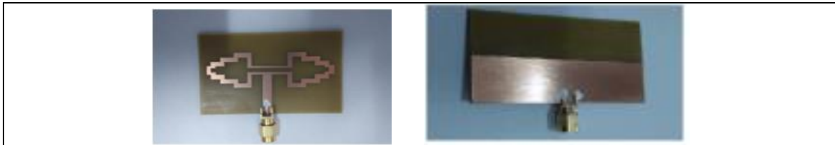
Fig 4: Fabricated dumbbell shape antenna with reduced ground plane (a) Top view (b) Bottom view
