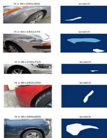
Fig.4 Plot of a subset from the full training dataset with their damage mask, image height included.
