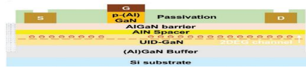
Fig-2: p-AlGa N gate enhancement-type HEMT [9].
