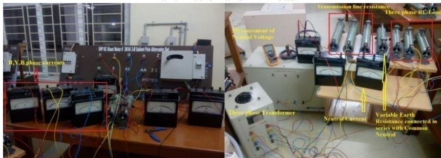
Figure 3.2 (b) Laboratory setup for Three Phase Four wire with Unbalanced Transmission and RL Load.
