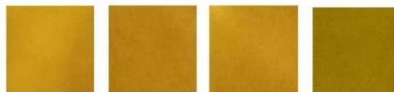
Figure 1 Typical transformer oil test images captured at different temperatures [15]
