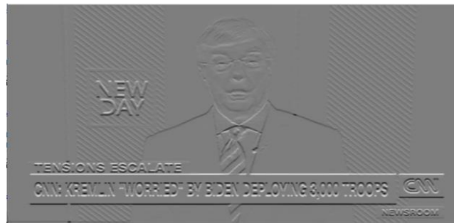
Fig. 3.3. Result after Sobel edge detection in x direction
