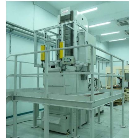
Vertical Broaching Machine EGIN RAS 10x1600x320
